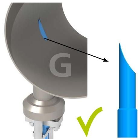
■ Use of a profiled piston on a tangential valve
