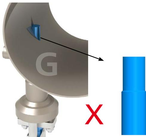
■ Use of a flat piston on a tangential valve
