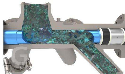
■ Profiled, rotating piston valve (Opened position)
